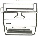
The input/output typewriter is used to print out messages and to send alphanumeric messages (letters and numbers) to the Communications Center and to other subscriber locations.
